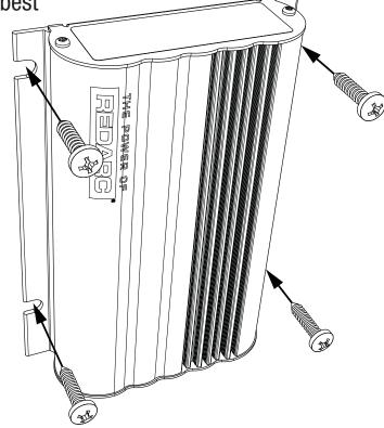
Figure 2.1.1 - Mounting the Charger
