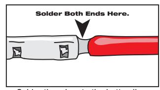
Solder the wires to the butt splice.
