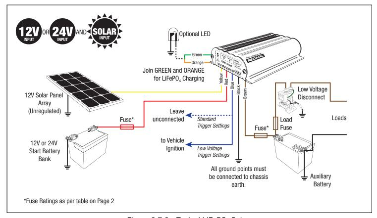
Figure 2.7.2 - Typical LiFePO<sub>4</sub> Setup
