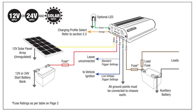
Figure 2.7.1 - Typical Lead Acid type Setup
