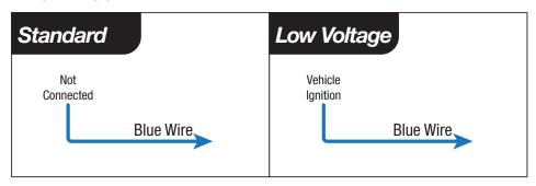
Figure 2.3.1 - Setting the Input Trigger Settings
